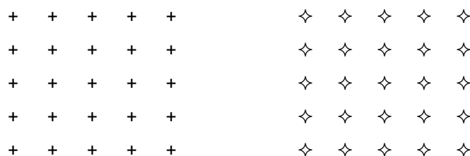
Figure A2.1 Two grid types suitable for systematic manual point counting of delta ferrite in duplex stainless steel
